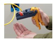
6. Wires will be seated and cut for a solid termination.
