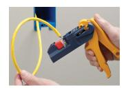
Insert jack in JackRapid front first with IDC slots facing blades of JackRapid.
